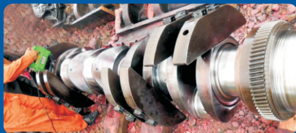
CRANK PIN MPI CRACK TESTING
