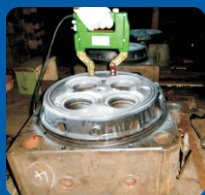
CYLINDER COVER MPI CRACK TEST
